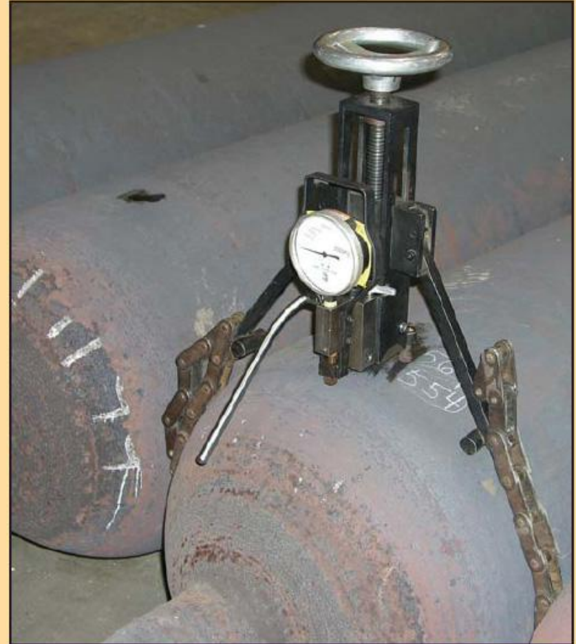
8. Hardness testing and other inspections confirm results of the heat-treating processes.
