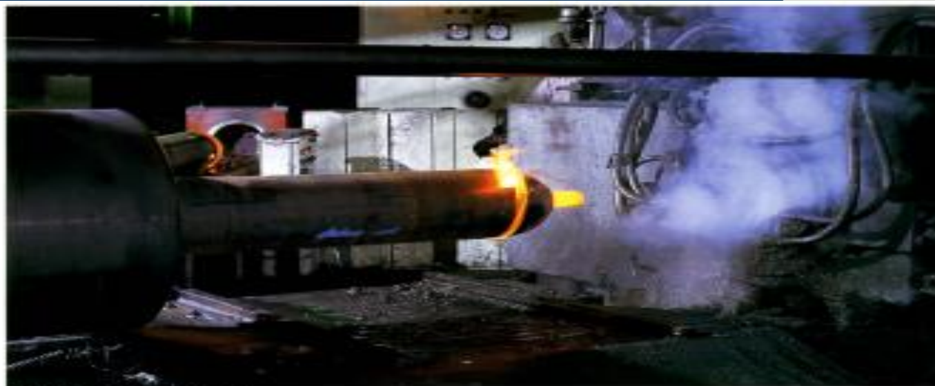
▲ 'Weslin' machine for top and forming
